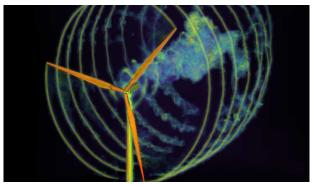
Blade-resolved simulations of wind energy applications are presented. Simulations of individual wind turbines are studied for accurate prediction and for learned simulation strategies to simulate full wind farms incorporating up to 100 wind turbines.
