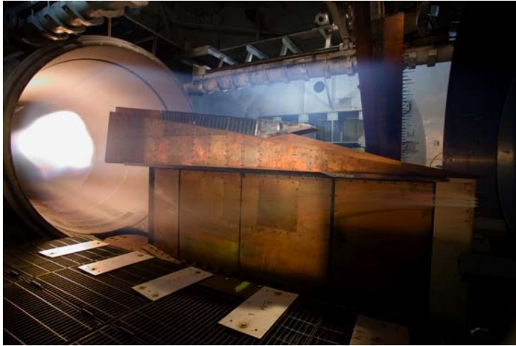
X-1 Engine Undergoes Testing in the 8ft Tunnel
